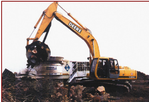
Materials being loaded into a tub grinder at the NCC Jersey City facility.
